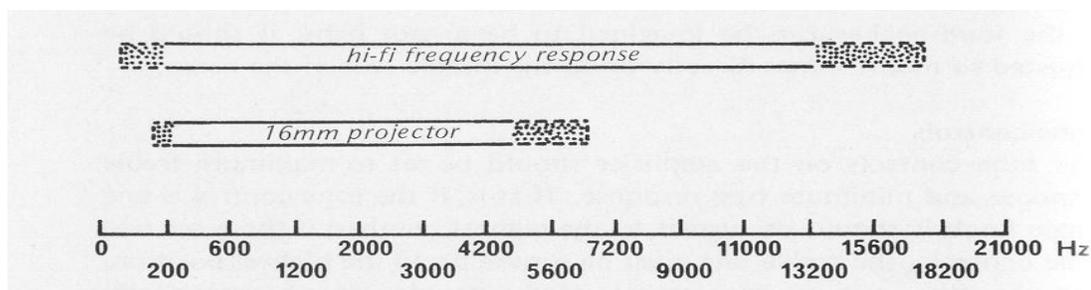
You can see how much of the frequency range is missing. You can never replace the missing frequencies, but you can partly compensate when you are setting your amplifier outputs. You don’t need much bass. But you
